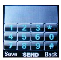
Touch icon with touch pen at standby status, the show the number simulate keyboard, use touch pen to press number, key in area no. and tell no. then press confirm key to dial
