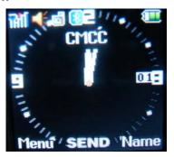
Press the power key for 2 seconds to turn on
